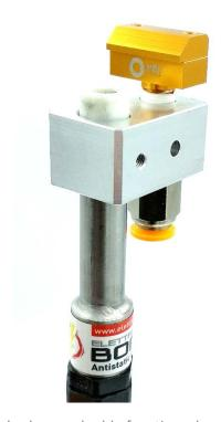
Compressed-air ionizing nozzles have a double function, cleaning the surface of interest and eliminate existing electrostatic charges. Ionizing nozzles are employed where installation conditions are critical, especially in confined spaces. Our ionizing nozzles can have multiple configurations and can be connected in series even in circular shape according to customer's needs.
