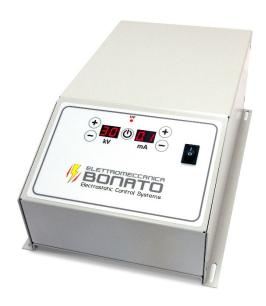
**ECG30** charge generator creates an adjustable high voltage between 0 to 30 KV and an also adjustable current between 0 and 3 mA. Its controls are very intuitive and thus easy to be used by the operator. Besides it can be remotely controlled by means of the remote control analogical function. It can have positive or negative charge on request and from 1 to 4 high voltage outputs.
