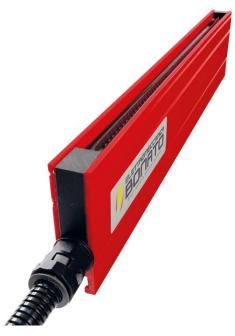
**CBR-LP-15** low profile electrostatically charging bars are designed to make a material adhere to a surface or two materials between them. These charging bars are connected to a generator, which creates (positive or negative) ions on bar's pointed edges by means of high voltage. Thus the material, passing through the bar and a reference mass, is pushed towards the mass itself, creating a temporary adhesion.
