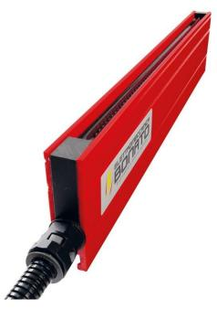
**CBR** electrostatically charging bars are designed to make a material adhere to a surface or two materials between them. These charging bars are connected to a generator, which creates (positive or negative) ions on bar's pointed edges by means of high voltage. Thus the material, passing through the bar and a reference mass, is pushed towards the mass itself, creating a temporary adhesion.
