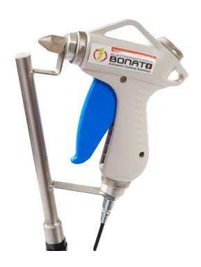
The antistatic gun AG-01, shockless, is a compressed air gun with a ions emitter nozzle. This allows that the air flow becomes ionized when you push the trigger and so able to eliminate the electrostatic charges, which are present on the surfaces where the trigger is directed. With this design the antistatic gun AG-01 is very effective in comparison with guns with internal ionization as well as very maneuverable and ergonimic.
