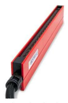
The **CBR-LP-10** low-profile charging bars are designed to make a material adhere to a surface or two materials adhere to each other. These charging bars are connected to a generator, which creates positive or negative ions on bar's pointed edges by means of high voltage. Thus, the material, passing through the bar and a ground mass, is pushed towards the mass itself, creating a temporary adhesion.
