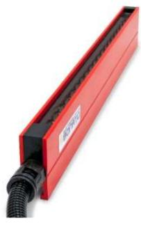
**CBR-LP-15** low profile electrostatically charging bars are designed to make a material adhere to a surface or two materials between them. These charging bars are connected to a generator, which creates (positive or negative) ions on bar's pointed edges by means of high voltage. Thus the material, passing through the bar and a reference mass, is pushed towards the mass itself, creating a temporary adhesion.
