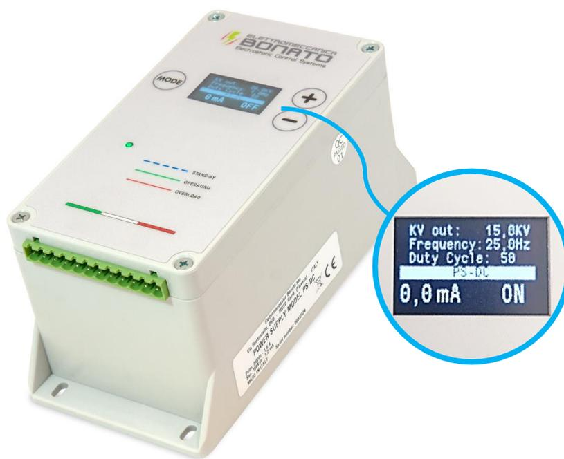
The PS-DC power supply unit generates pulsed voltage that can be adjusted between 0 and 15 KV, with a frequency that can be adjusted from 0.5 to 25Hz. The duty cycle can also be adjusted from 20/80 to 80/20 positive/negative.
